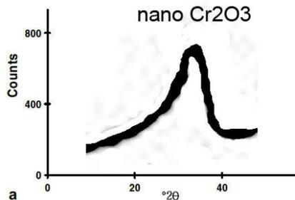
Fig. 3. XRD analysis of Cr<sub>2</sub>O<sub>3</sub> nanoparticles.
