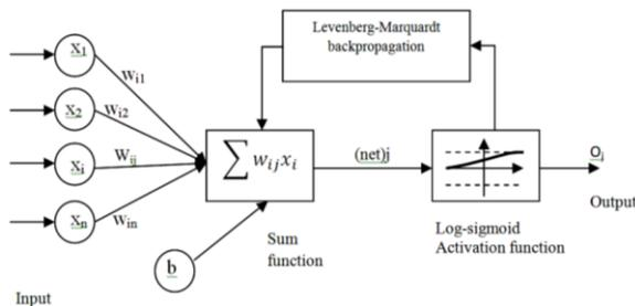
Fig. 4. Architecture of applied neural network.
