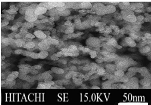
Fig. 2. SEM micrograph of Cr<sub>2</sub>O<sub>3</sub> nanoparticles.
