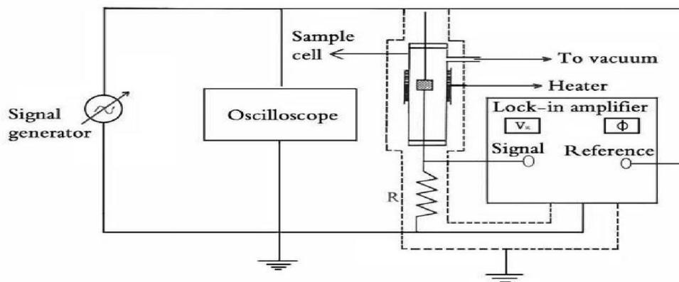
**Fig. (1) Block diagram of the experimental arrangement for measuring A.C. Properties by using a lock-in amplifier.**
