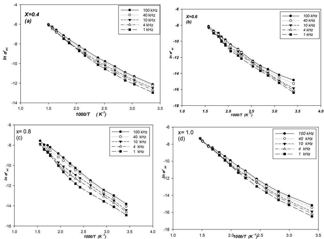
Fig. (4 a-d) Temperature dependence of  $\ln \sigma'_{ac}$  at five different frequencies ( $f = 1, 4, 10, 40, 100$  kHz) for all samples.
