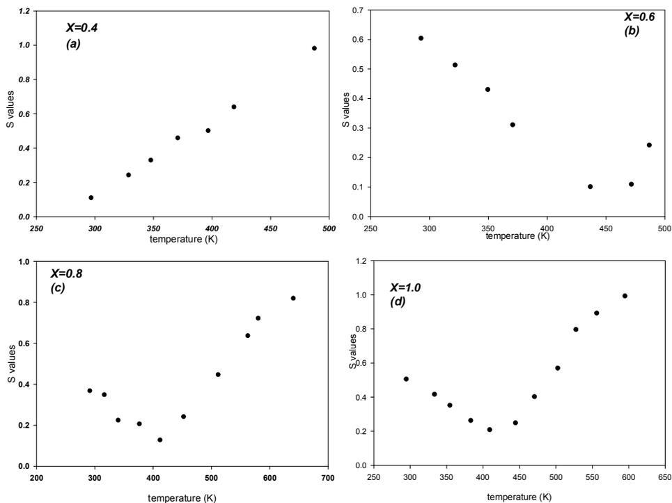
Fig. (5 a-d) Temperature dependence of the exponent  $s$  for different compositions of  $Ni_{1.7}Cd_{0.3}Fe_{2-x}Al_xO_4$ .
