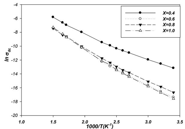
Fig (1) the variation of  $\ln\sigma_{dc}$  vs.  $10^3/T(K^{-1})$  for the samples  $Ni_{0.7}Cd_{0.3}Fe_{2-x}Al_xO_4$ .
