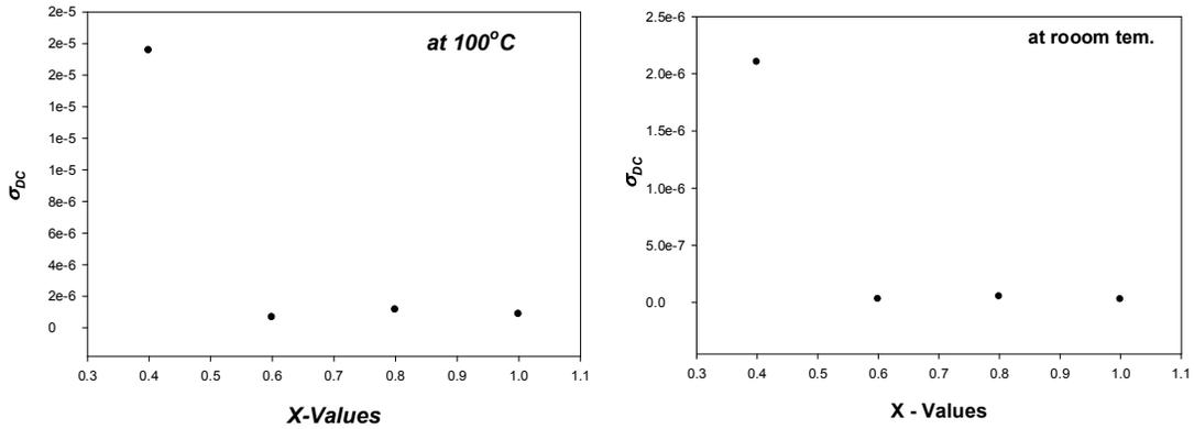
Fig (2) the variation of dc electrical conductivity as a function of composition (x) at 100°C and room temperature
