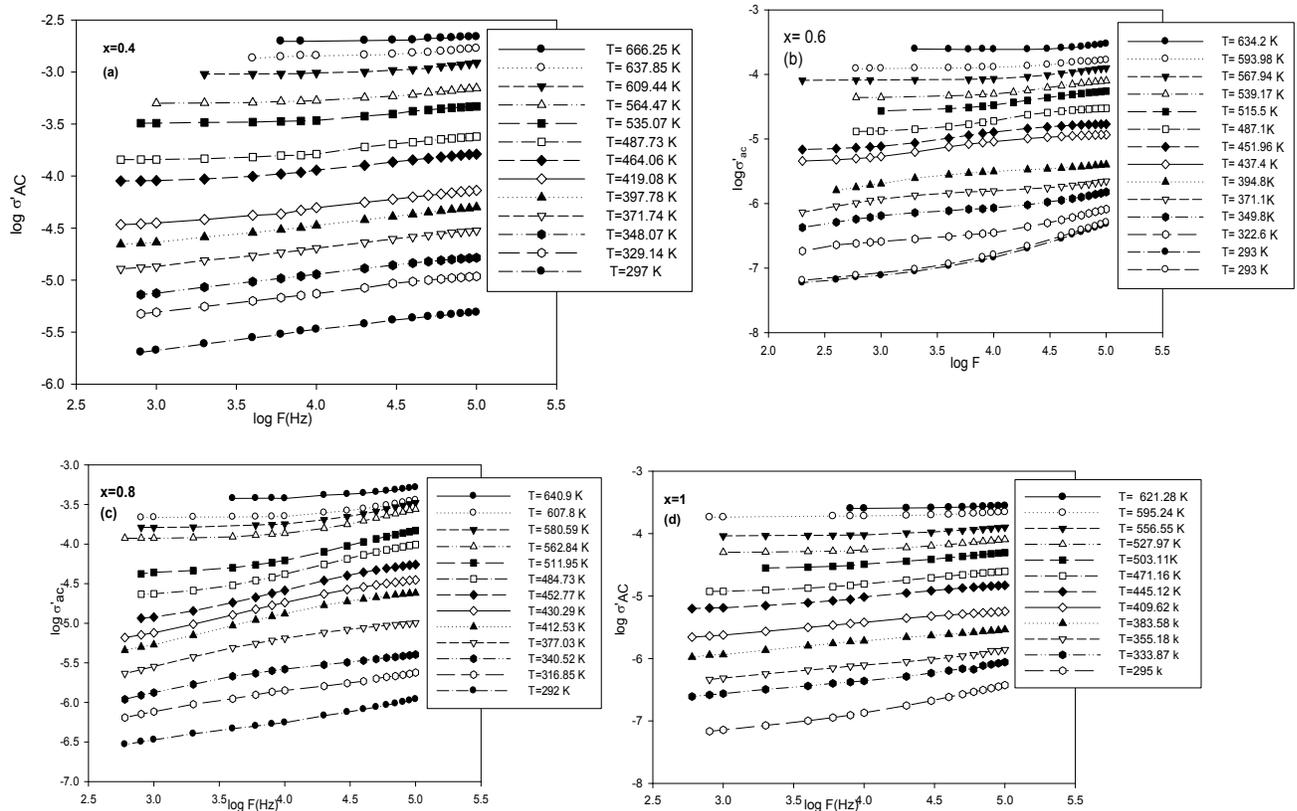
Fig. (3 a-d) the variation of  $\log \sigma_{ac}$  with the frequency as  $\log f$  at different temperature for all studied samples.
