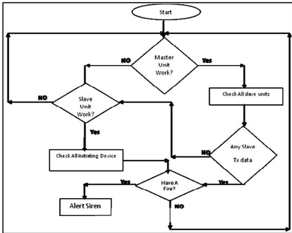
Figure 5. Wireless Intelligent Fire Alarm system flowchart operation
