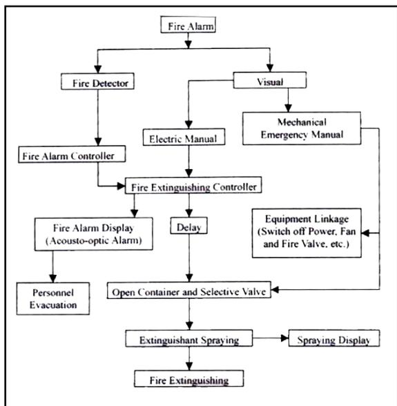
Figure 1. Fire Alarm system overview
