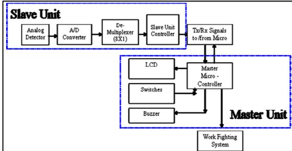
Figure 4. Wireless Intelligent Fire Alarm system block diagram
