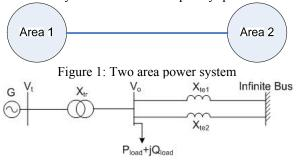
Figure 2: A single machine infinite bus power system
