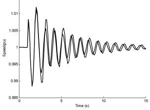
Figure 6: Speed response following three phase short circuit in bus 1 in the nominal operating condition. (Solid: MRAS-PSS; Dashed: GA-PSS)
