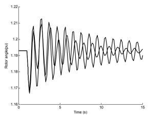
Figure 7: Rotor angle response following three phase short circuit in bus 1 in the heavy operating condition. (Solid: MRAS-PSS; Dashed: GA-PSS)
