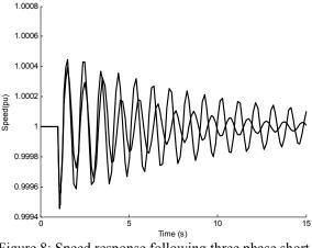
Figure 8: Speed response following three phase short circuit in bus 1 in the heavy operating condition. (Solid: MRAS-PSS; Dashed: GA-PSS)
