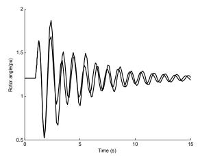
Figure 5: Rotor angle response following three phase short circuit in bus 1 in the nominal operating condition. (Solid: MRAS-PSS; Dashed: GA-PSS) 1.015r
