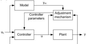
Figure 3: Block diagram of model reference adaptive system
