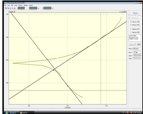
**Fig-9 Polarization curve for (Al-4%Zn-0.5%Sn) alloy**
