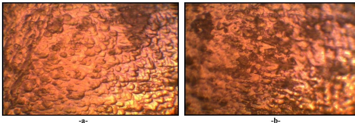
**Fig-12 a: The microstructure of (Al – 4% Zn -0.4%Sn)alloy after immersion, 400X**
