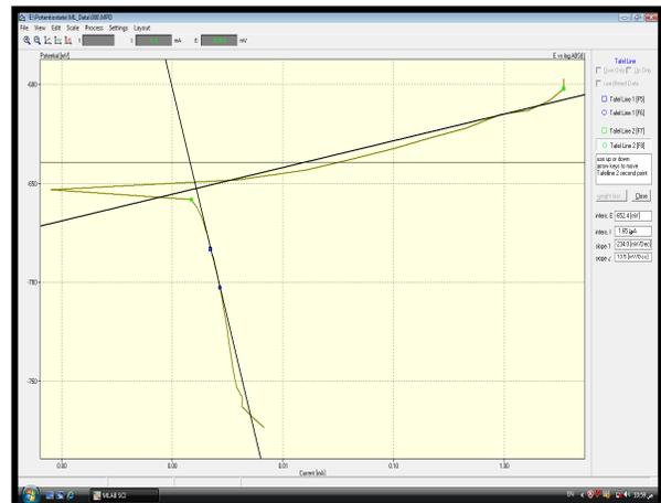
**Fig-7 Polarization curve for (Al-4%Zn) alloy**
