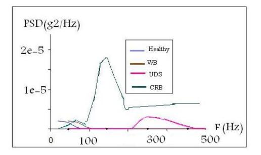
Figure 4. Power Spectral Density results of starter motor on healthy and fault conditions
