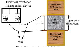
Fig. 1. Schematic of resistivity test setup
