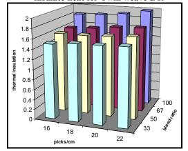
Fig (8): The effect of number of picks per cm and the ratio of polyester hollow fibers upon the ability of produced fabrics to insulate heat for Twill weave 3/1.
