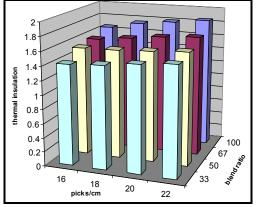
Fig (6): The effect of number of picks per cm and the ratio of polyester hollow fibers upon the ability of produced fabrics to insulate heat for Twill weave 2/1.
