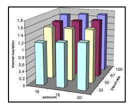
Fig (5): The effect of number of picks per cm and the ratio of polyester hollow fibers upon the ability of produced fabrics to insulate heat for Plain weave 1/1.
