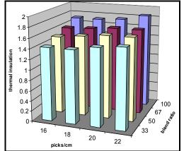
Fig (7): The effect of number of picks per cm and the ratio of polyester hollow fibers upon the ability of produced fabrics to insulate heat for Twill weave 2/2.
