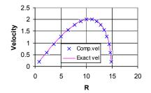
Figure 9: Comparison of computed and analytical velocity distributions over the boundary of a Joukowski aerofoil using first 16 values of 32 boundary elements with constant element approach r = 7.5, a = 0.1, c = 0.1 and Ma = 0.7.
