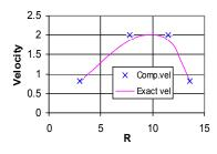
Figure 5: Comparison of computed and analytical velocity distributions over the boundary of a Joukowski aerofoil using first 4 values of 8 boundary elements with constant element approach for r = 7.5, a = 0.1, c = 0.1 and Ma = 0.7.
