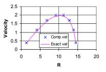
Figure 8: Comparison of computed and analytical velocity distributions over the boundary of a Joukowski aerofoil using last 8 values of 16 boundary elements with constant element approach r = 7.5, a = 0.1, c = 0.1 and Ma = 0.7.
