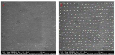
Figure (1):a. scanning photomicrograph of Beautifil II specimen after exposure to coffee, b. image analysis divided the scanning photomicrograph into points.
