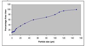
Fig. 1. Illustration of cement particles' distribution.
