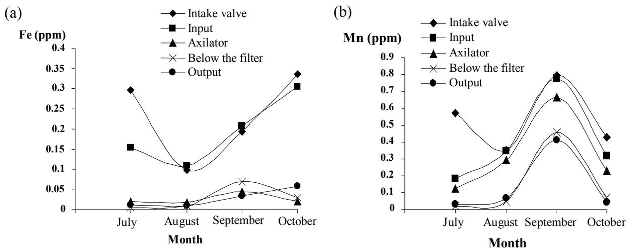
Figure 2. Concentration changes of iron and manganese [Iron, (a)] and [Manganese, (b)].
