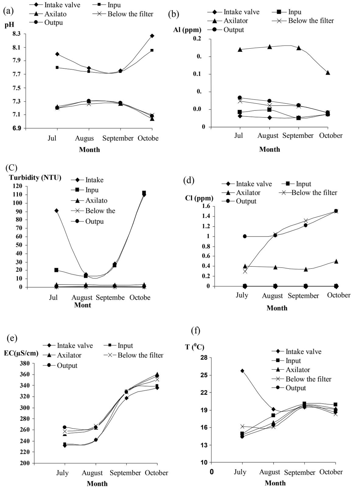
Figure 3. Quality Parameters in water treatment plant include [pH, (a)], [Mean concentration of aluminum, (b)], [Mean turbidity, (c)], [Mean concentration of chlorine, (d)], [Electrical conductivity, (e)] and [Temperature, (f)].
