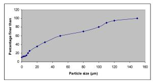
Fig. 1. Illustration of cement particles' distribution.
