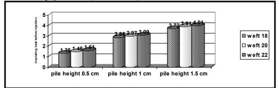
Fig. (12):Effect of pile height and number of picks/cm on thermal insulation for fabrics which produced from
