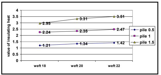
Fig. (7):Effect of number of picks/cm on thermal insulation for fabrics which produced from 30% cotton and 70% polyester fibers (after treatment)
