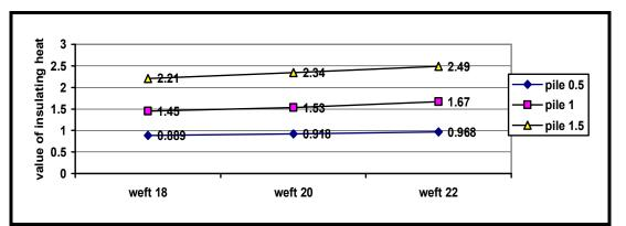
Fig. (5):Effect of number of picks/cm on thermal insulation for fabrics which produced from 100% cotton fibers (after treatment)
