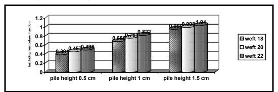
Fig. (2):Effect of pile height and number of picks/cm on thermal insulation for fabrics which produced from 70% cotton and 30% polyester fibers (before treatment)
