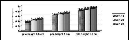
Fig. (1):Effect of pile height and number of picks/cm on thermal insulation for fabrics which produced from 100% cotton fibers (before treatment)
