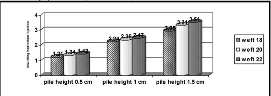
Fig. (11):Effect of pile height and number of picks/cm on thermal insulation for fabrics which produced from 30% cotton and 70% polyester fibers (after treatment)
