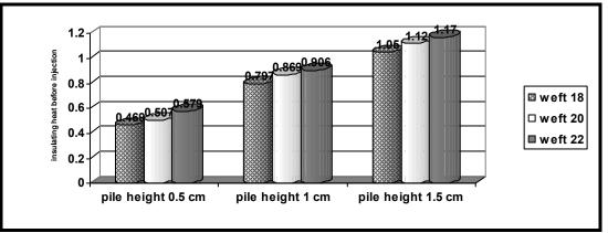
Fig. (3):Effect of pile height and number of picks/cm on thermal insulation for fabrics which produced from 30% cotton and 70% polyester fibers (before treatment)
