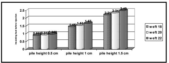
Fig. (9):Effect of pile height and number of picks/cm on thermal insulation for fabrics which produced from 100% cotton fibers (after treatment)
