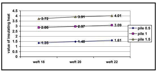
Fig. (8):Effect of number of picks/cm on thermal insulation for fabrics which produced from 100% polyester fibers (after treatment)
