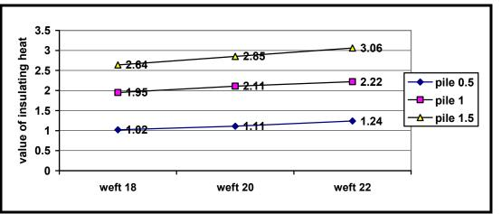
Fig. (6):Effect of number of picks/cm on thermal insulation for fabrics which produced from 70% cotton and 30% polyester fibers (after treatment)
