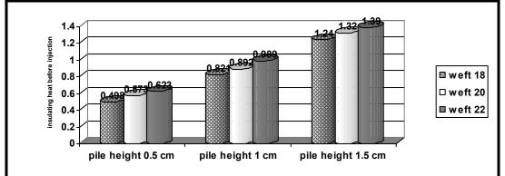
Fig. (4):Effect of pile height and number of picks/cm on thermal insulation for fabrics which produced from 100% polyester fibers (before treatment)
