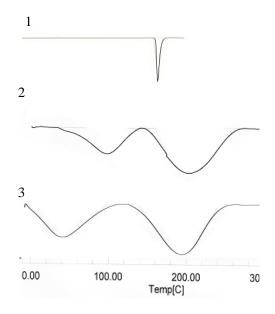
Figure 3: DSC thermograms of (1) Paracetamol, (2) Indion 204 and (3) Paracetamol-resinate complex
