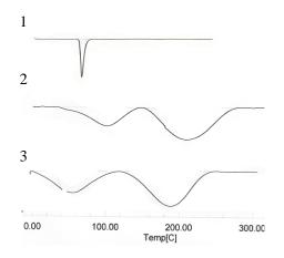
Figure 4: DSC thermograms of (1) Ibuprofen, (2) Indion 204 and (3) Ibuprofen resinate-complex
