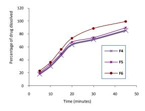
Figure 8: Dissolution profile of Paracetamol from prepared chewable tablet formulae
