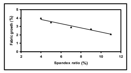
Figure 4: Effect of spandex ratio on fabric growth
