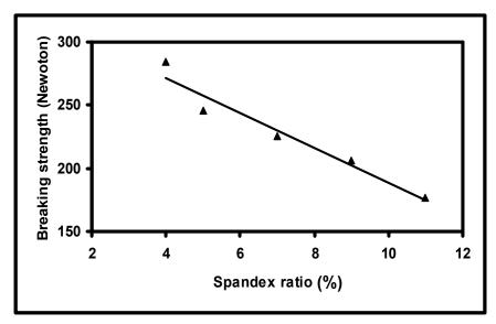
Figure 1: effect of spandex ratio on fabric breaking strength
