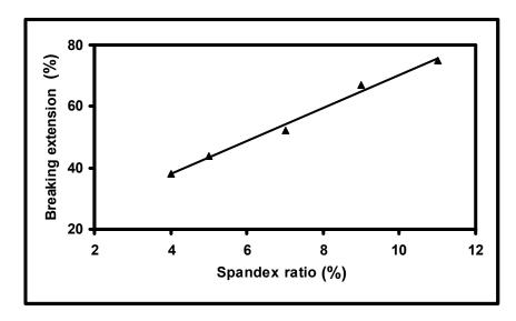
Figure 2: Effect of spandex ratio on fabric breaking extension
