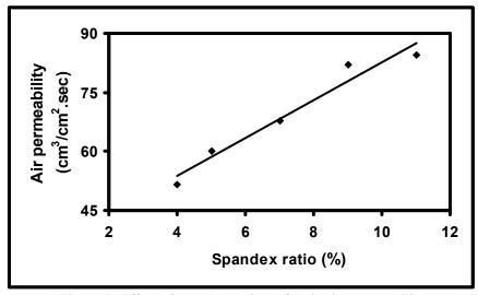
Figure 5: Effect of spandex ratio on fabric air permeability
