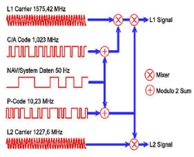
Fig 2.0. GPS Signal structure [16] Source: Kowoma (2005)
