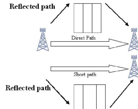
Figure 7. Inter Symbol Interference
