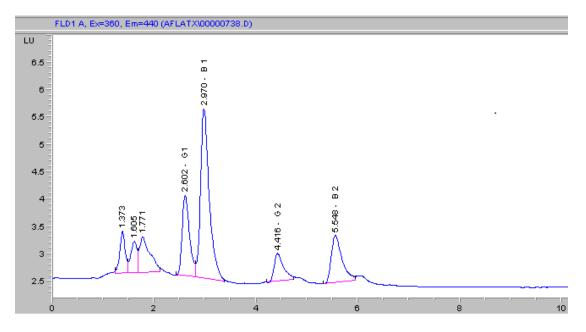
Figure (2): High Performance Liquid Chromatogram of a standard of aflatoxins (AFG<sub>1</sub>,AFB<sub>1</sub>, AFG<sub>2</sub> and AFB<sub>2</sub>)
