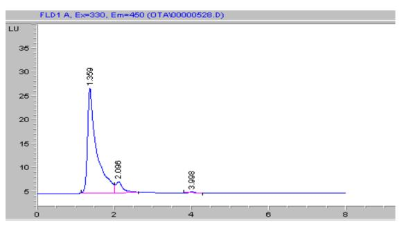
Figure (3): High Performance Liquid Chromatogram of a negative sample of aflatoxins (AFG<sub>1</sub>,AFB<sub>1</sub>, AFG<sub>2</sub> and AFB<sub>2</sub>)
