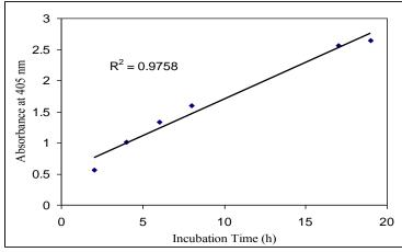
Figure 12. Relationship between incubation time and absorbance of yellow color liberated by a constant amount of the clear supernatant of a selected isolate using chromogenic assay of PLC activity.
