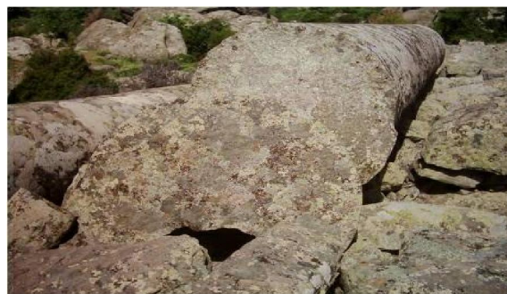
Figure 2. A Sample Exposed to Deterioration By Acid From The Research Field: The Column in Koçali Quarry
