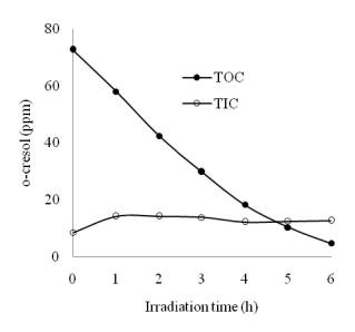
Fig.5 the amount of TOC and TIC during photodegradation of o-cresol under UV irradiation, initial condition; o-cresol concentration = 100 ppm, ZnO = 2.5g/L and pH = 7.37
