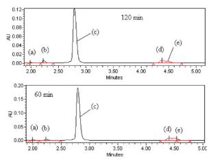
Fig. 6 selected UPLC chromatograms of o-cresol under UV irradiation that shows (a) 2methylresorcinol, (b) 2,5-hydroxybenzaldehyde and (c) unknown (d) salicylaldehyde as intermediates and (e) o-cresol. Concentration of o-cresol= 50ppm at 60min
