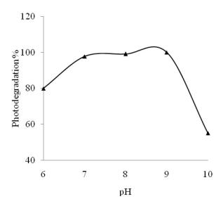
Fig.4. Photodegradation of o-cresol at variation initial pH under UV irradiation, initial condition, o-cresol concentrations = 100ppm, photocatalyst = 2.5g/L, during 6h.
