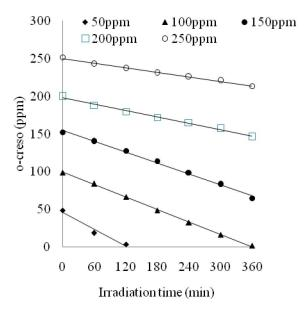
Fig. 3 Effect of o-cresol concentration on photodegradation under UV irradiation, initial condition: photocatalyst concentration = 2.5 g/L, and pH = 7.37
