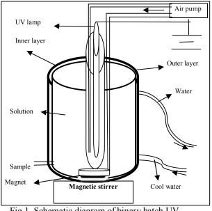
Fig.1. Schematic diagram of binary batch UV photoreactor
