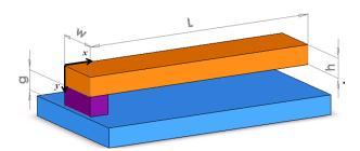
Fig.1. Schematic representation of a cantilever nanobeam
