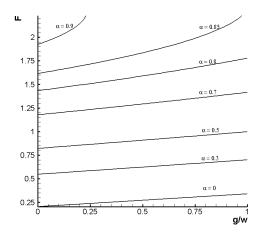
Fig.2. Effect of fringing filed and intermolecular force on the shear force at the fixed end of cantilever nano-beam when  $\beta$ =0.2
