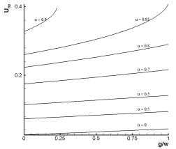
Fig.4. Effect of fringing filed and intermolecular force on the tip deflection of cantilever nano-beam when  $\beta=0.2$
