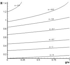
Fig.3. Effect of fringing filed and intermolecular force on the bending moment at the fixed end of cantilever nano-beam when  $\beta$ =0.2
