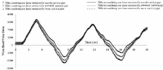
Fig 5: Changes of water head versus time in middle of the pipe considering the pipe material in the two cases, i.e. with and without considering nonlinear terms.
