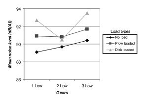
Figure 1. Mean noise level in different gears for tractor without cabin.
