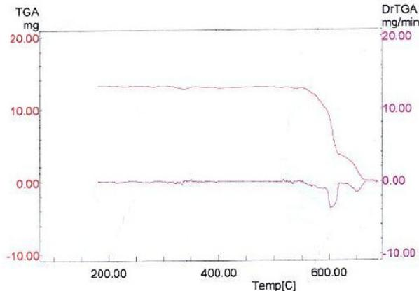
Fig. (2): TGA – DTA pattern of mineral fibers
