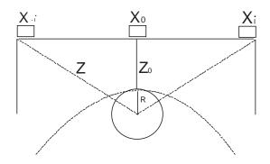
Fig. 1, hyperbolic signature spread due to buried cylinder
