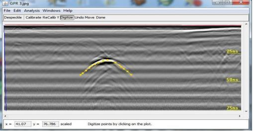
Fig. 3, digitized radar scan
