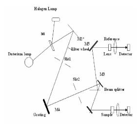
Figure 3: Block Diagram of UV-Visible Spectrometer
