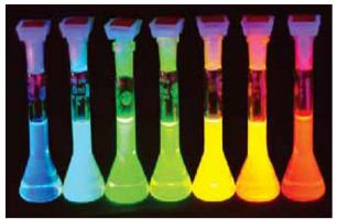
Figure 1: Fluorescence in different-sized CdSe quantum-dots
