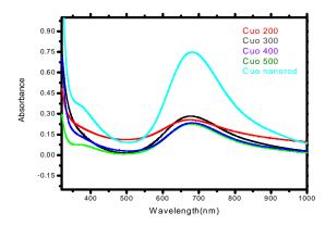
Figure 5: UV-Visible absorption spectrum of CuO nanocrystals
