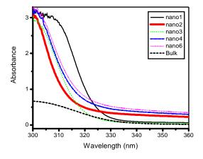
Figure 4: UV-Visible absorption spectrum of ZnS quantum dots
