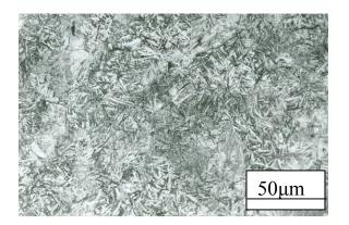
Fig. 4 Microstructure of the screw conveyor
