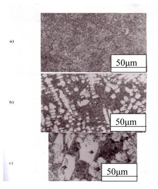
Fig. 6 Microstructure at the top surface of the weld metal using a) Electrode A, b) Electrode B, and Electrode C
