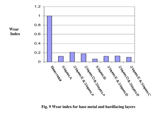
Fig. 9 Wear index for base metal and hardfacing layers
