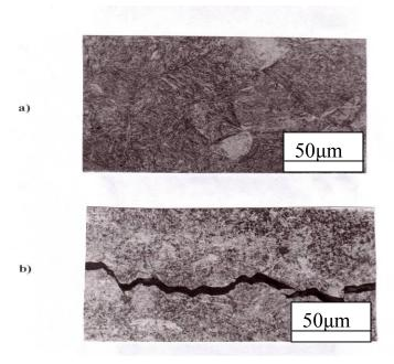
Fig. 5 Microstructure at the HAZ of the base metal a) Crack free specimen,
