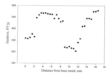
Fig. 8 Hardness distribution along the base metal, HAZ and hardfacing material using electrode E and three layer of electrode A.
