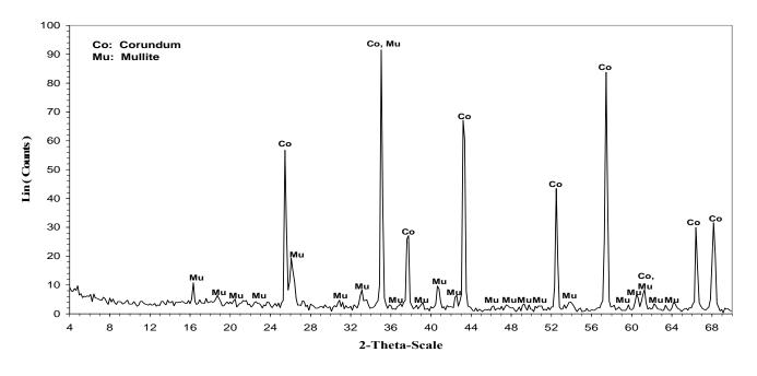
Fig. (1): XRD Pattern of Calcined Bauxite
