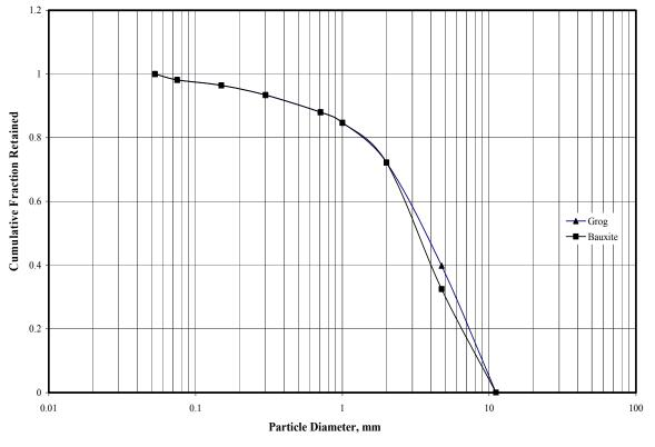
**Fig. (3): Particle Size Distribution of Aggregates**
