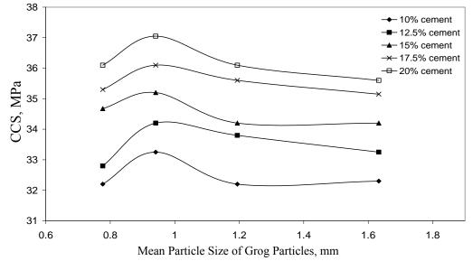
Fig. (13): Effect of Mean Particle Size of Grog Aggregates Containing Different Cement Percents on the Cold Crushing Strength of Mixes
