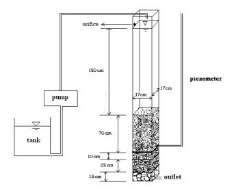
Fig 1. Schematic of filter
