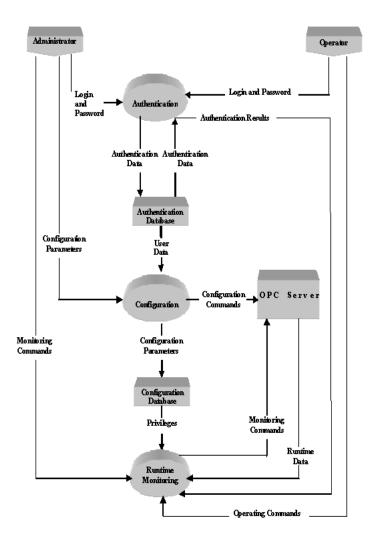
Figure 2. First level DFD of the system
