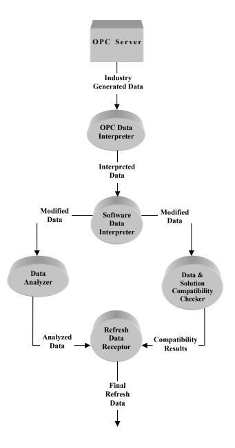
Figure 3. Second level DFD of the system
