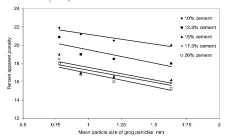
Fig. (8): Effect of Amount of Cement Used and Mean Particle Size of Aggregate on Percent Apparent Porosity for Bauxite Based Mixes
