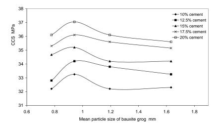
Fig. (13): Effect of Amount of Cement Used and Mean Particle Size of Aggregate on the Cold Crushing Strength of Grog Based Mixes
