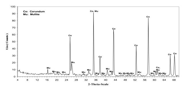
Fig. (2): XRD Pattern of Calcined Bauxite
