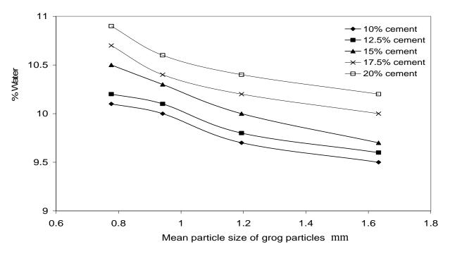
Fig. (5): Effect of Amount of Cement Used and Mean Particle Size of Aggregate on Water Consumption for Grog Based Mixes
