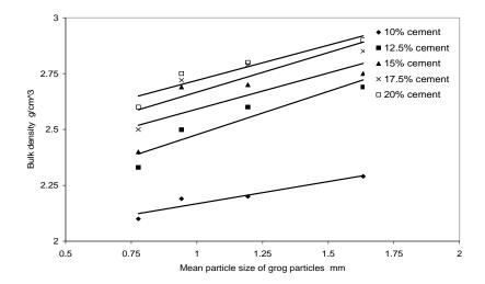
Fig. (11): Effect of Amount of Cement Used and Mean Particle Size of Aggregate on the Bulk Density of Grog Based Mixes
