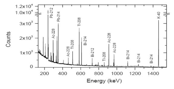
Figure 2: A typical gamma-ray spectrum showing important identified photo-peaks and their associated Radionuclides
