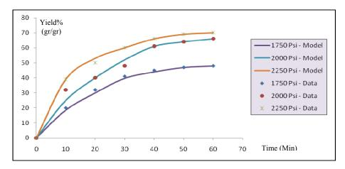
Fig 2. Effect of pressure on the extraction yield of oil at T=328 K and dp=0.12 mm
