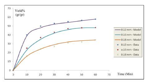
Fig 4. Effect of particle size on the extraction yield of oil at P= 2250 Psi and T= 328 K
