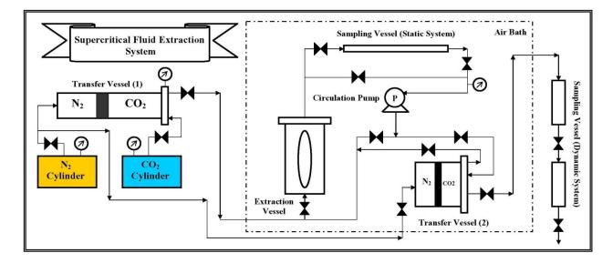
Fig1. Schematic diagram of the Supercritical Fluid Extraction System (SCFE) for Extraction of oil from canola seed with supercritical carbon dioxide
