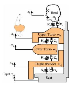
Figure 1: Biomechanical Boileau and Rakheja 4-DOF model.
