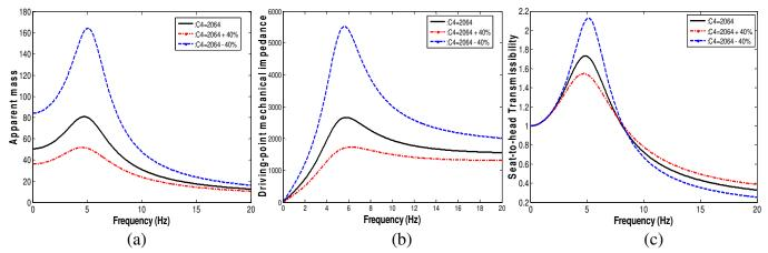
**Figure 4**: Effect of damping coefficient on the biodynamic response behaviors (Analytic Results) ((a) STHT, (b) DPMI and (c) APMS)
