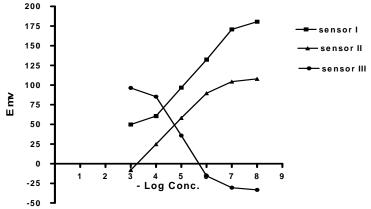
Figure (2): Profile of the potential in mV vs. –log concentration of lisinopril in M using the three studied electrodes: Lisinopril-bathophenanthroline-iron-PVC classical (sensor I), Lisinopril-bathophenanthroline-iron-PVC coated wire (sensor II) and hydroxypropyl &-CD-Tecoflex graphite (sensor III)
