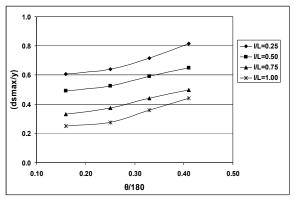
Figure 12. Effect of location on relative maximum depth of scour
