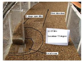
Figure4. Scour pattern at the end of a test
