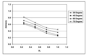
Figure 10. Effect of wing length on relative maximum depth of scour
