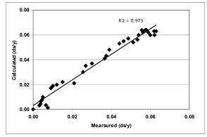
Figure13. Comparison of measured and predicted scour depth
