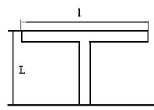
Figure2. A T-shape spur dike (Plan)
