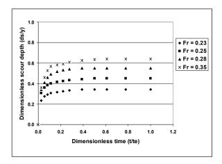
Figure5. Time development of scour for different Froude number
