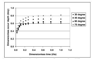
Figure11. Time development of scour for different locations
