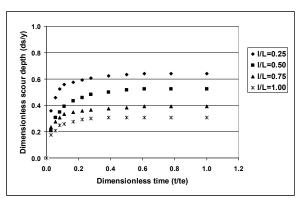
Figure9. Time development of scour for different wing lengths
