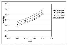
Figure8. Effect of length on relative maximum depth of scour
