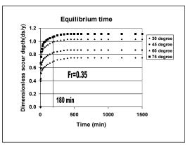
Figure3. Equilibrium time in the different position for a T-shape spur dike
