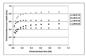
Figure7. Time development of scour for different lengths
