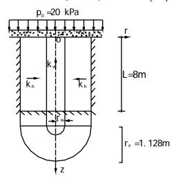
Figure 4 the sketch of single sand drain
