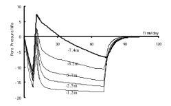
Figure 9b Sand Drain Element pore water pressure
