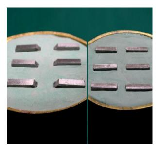
Fig. 1: Stainless steel strips with butt and 45<sup>0</sup> bevel embedded in lower half of flask.
