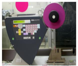
Fig.6: Test for Impact strength under progress using Ceast, Resil Impactor machine
