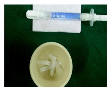
Fig.4: Glass fibers soaked in silane coupling agent
