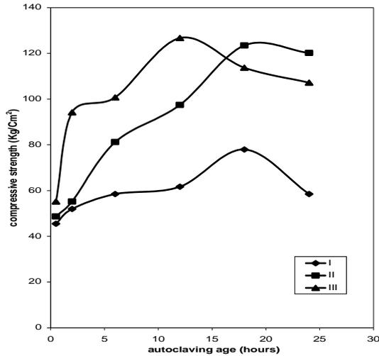
Fig.(1): Compressive strength (Kg/cm<sup>2</sup>) of Mixes I,II and III at various autoclaving ages.
