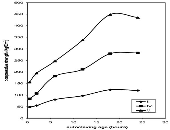
Fig.(2): Compressive strength (Kg/cm<sup>2</sup>) of Mixes II, IV and V at various autoclaving ages.
