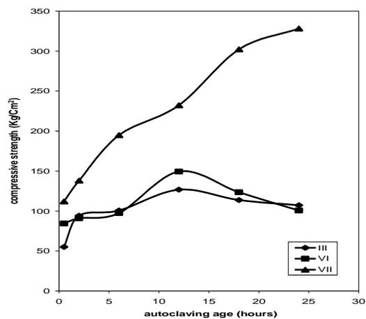
Fig.(3): Compressive strength (Kg/cm<sup>2</sup>) of Mixes III, VI and VII at various autoclaving ages.
