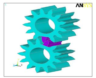
Figure 1. The thorough model of the hydraulic pump gears in 955 combine
