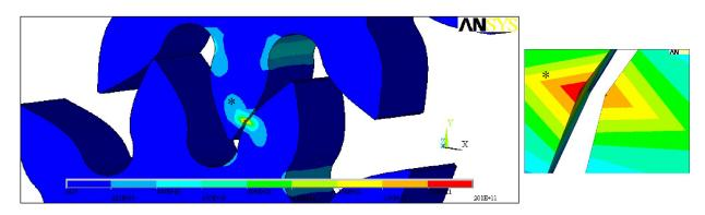
Figure 5. The stresses on the contact region of the engaged teeth due to the tensional loading
