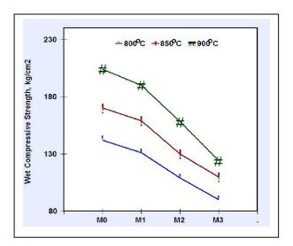
Fig. (2): Dry and wet compressive strength of fired briquettes as a function of OBM content as well as firing temperatures.
