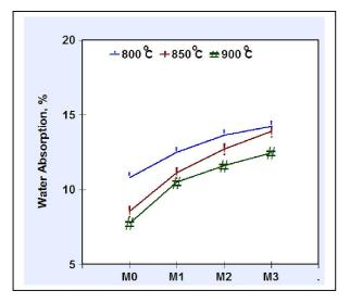
Fig. (1): Water absorption and bulk density as a function of OBM waste content as well as firing temperatures.
