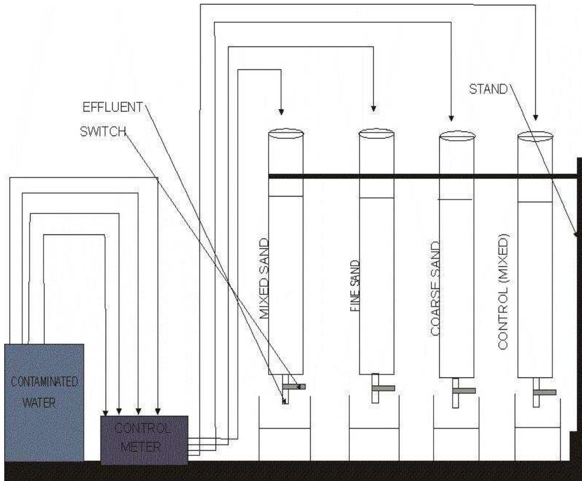
Fig. 1. Schematic diagram of the experiment with 4 columns.
