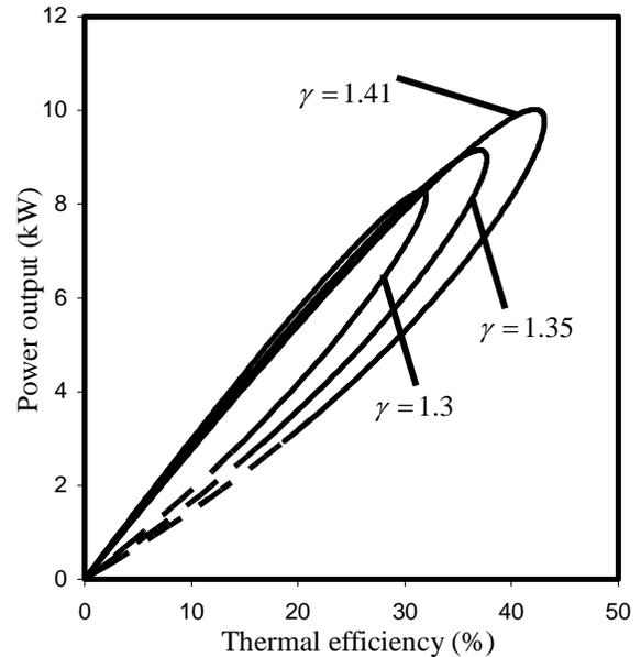
Figure 4. Effect of specific heat ratio on the variation of the output power with thermal efficiency
