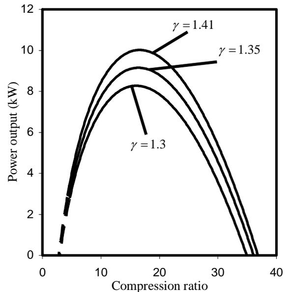
Figure 2. Effect of specific heat ratio on the variation of the output power with compression ratio
