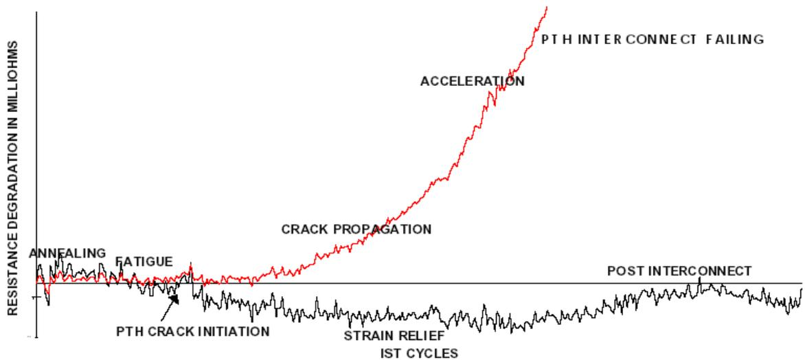
Figure 6. Resistance Degradation of the PTH Interconnect During an Accelerated Interconnect Stress Testing adopted from IPC-TM-650 [9]
