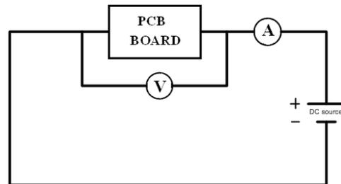
Figure 7. The Circuit for IST thermal cycling
