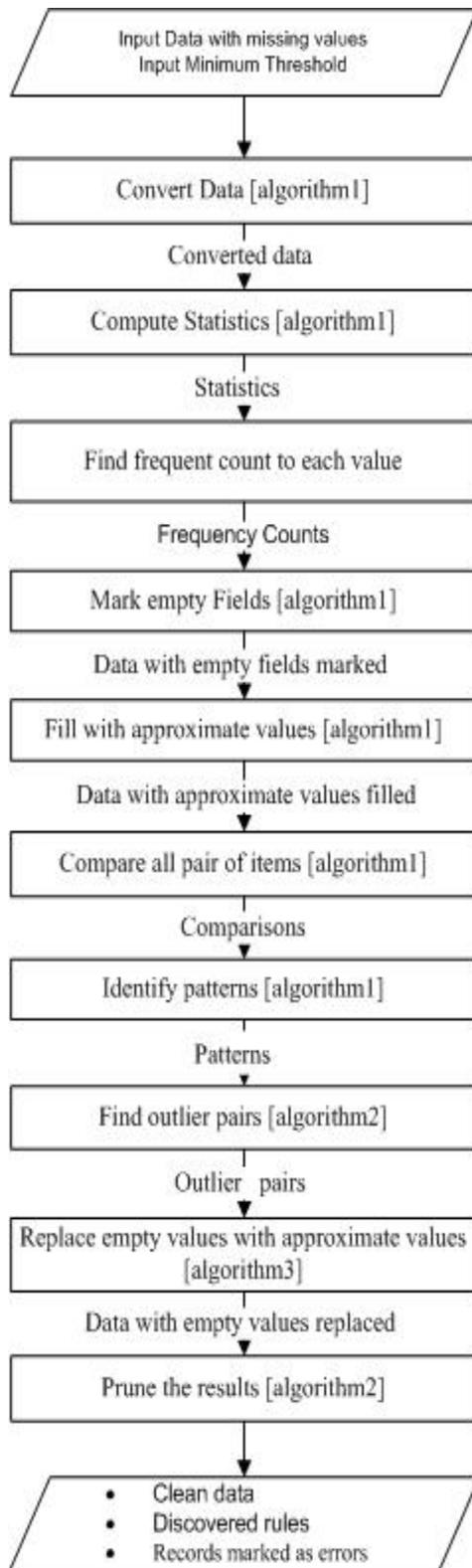
Fig. 1 Dataflow diagram for applying ordinal association rules for cleansing data with missing values.
