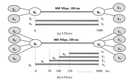
Fig.1 Network topology used in the simulations with active periods of the flows
