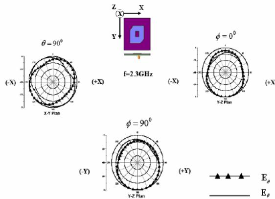
Figure 2. Field measurements of the proposed OD antenna with NIQ/Cu patch on FR4 substrate at thickness of 1.6mm
